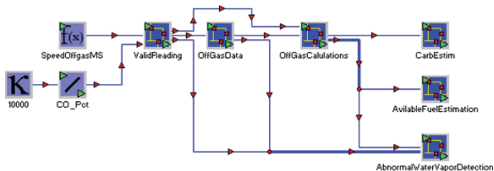
Figure 4. Off Gas Control Module
