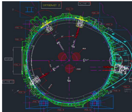
Fig. 5 – EAF Layout with the new burner
