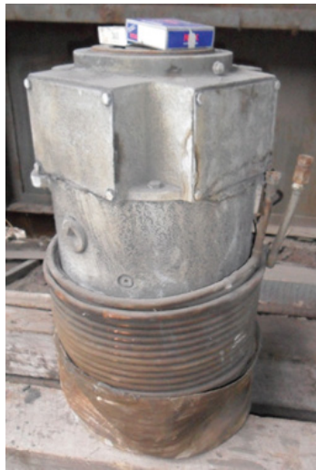
Figure (2). Original DC Motor with water-cooled coil in the center.
