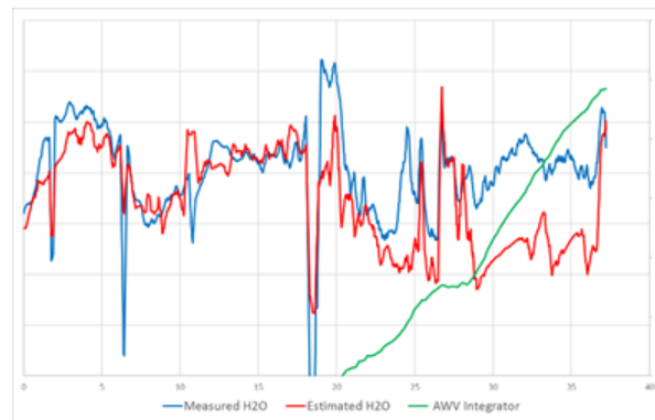
Fig. 15 – Detection of a Water Leak
